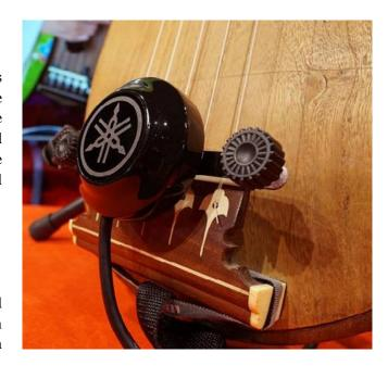
Figure 7: The device called "Real Sound Reproducer" attached to the bridge of the instrument. Photo: Hamamatsu Museum of Musical Instruments
