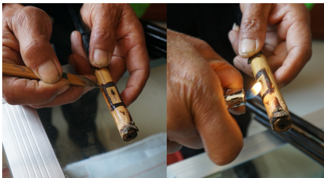
Fig. 3. The craftsmanship technology of a Wa Gourd sheng : fixing a reed with black wax.
