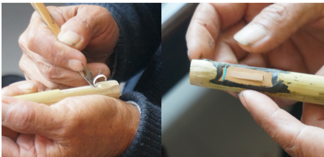
Fig. 2. The musical-instrument maker Mr. Tian Kaizheng fitting a reed of "Bi Lag Leen" into a reed window.
