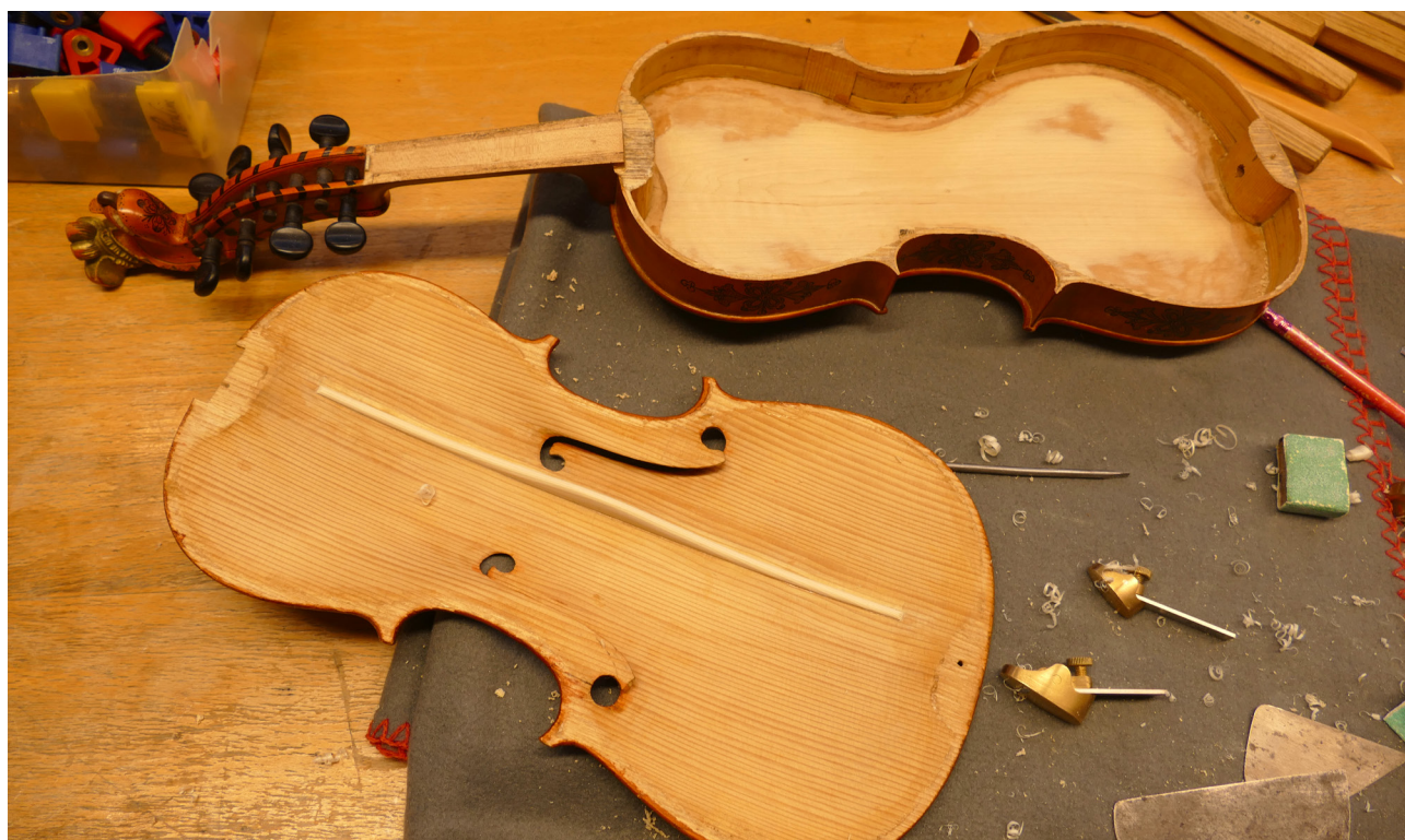
Fig. 5. Thinning an overly thick bottom patch and replacing a non-original bass bar of a Hardanger fiddle by Gunnar Røstad, 1912.
