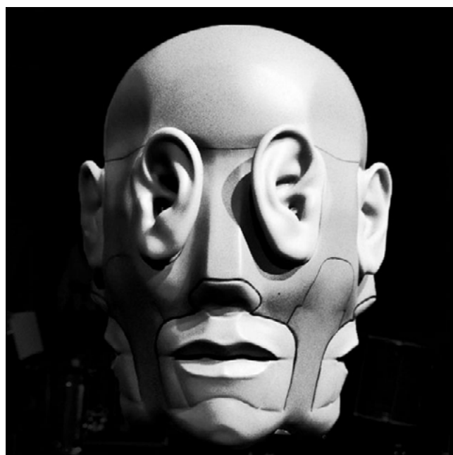
Figure 1: “The Head” – a four-channel 3D-audio microphone rig.
