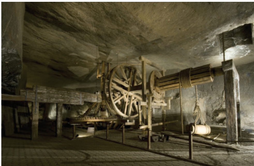
A horse mill (called the “Polish mill” with a horizontal shaft, the oldest and the largest winding gear in the museum collection, 17 th c.
